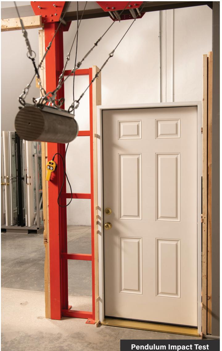
Pendulum Impact Test
