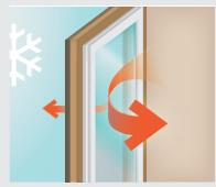
In cold weather, Low-E glass can help reduce the loss of heat by reflecting the heat back inside the home.
